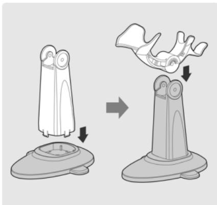
① Fit the bracket into the base to lock the bracket to the base.
