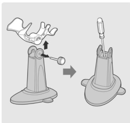
① Release the knob to remove the scanner holder.
