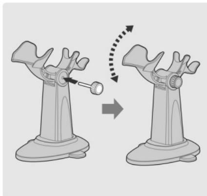
① Insert the angle adjustment knob. Turn the knob clockwise to secure the scanner holder to the bracket.
